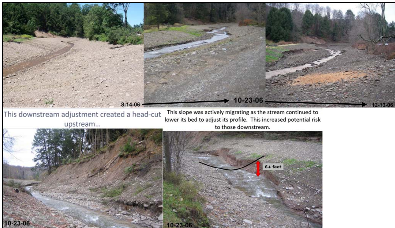
Figure 2: The photos show the stream channel evolution for inappropriate sized stream. Large amounts of sediment are easily moved during small events impacting water quality.
